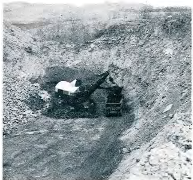
In operation at the mine since 1937, this electric loading shovel has a 3-cu-yd dipper.
