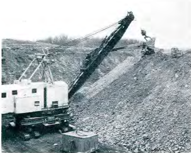
This 15-cu-yd electrically powered shovel has been in service since 1937. It has a 96-ft boom and a 58-ft stick.
